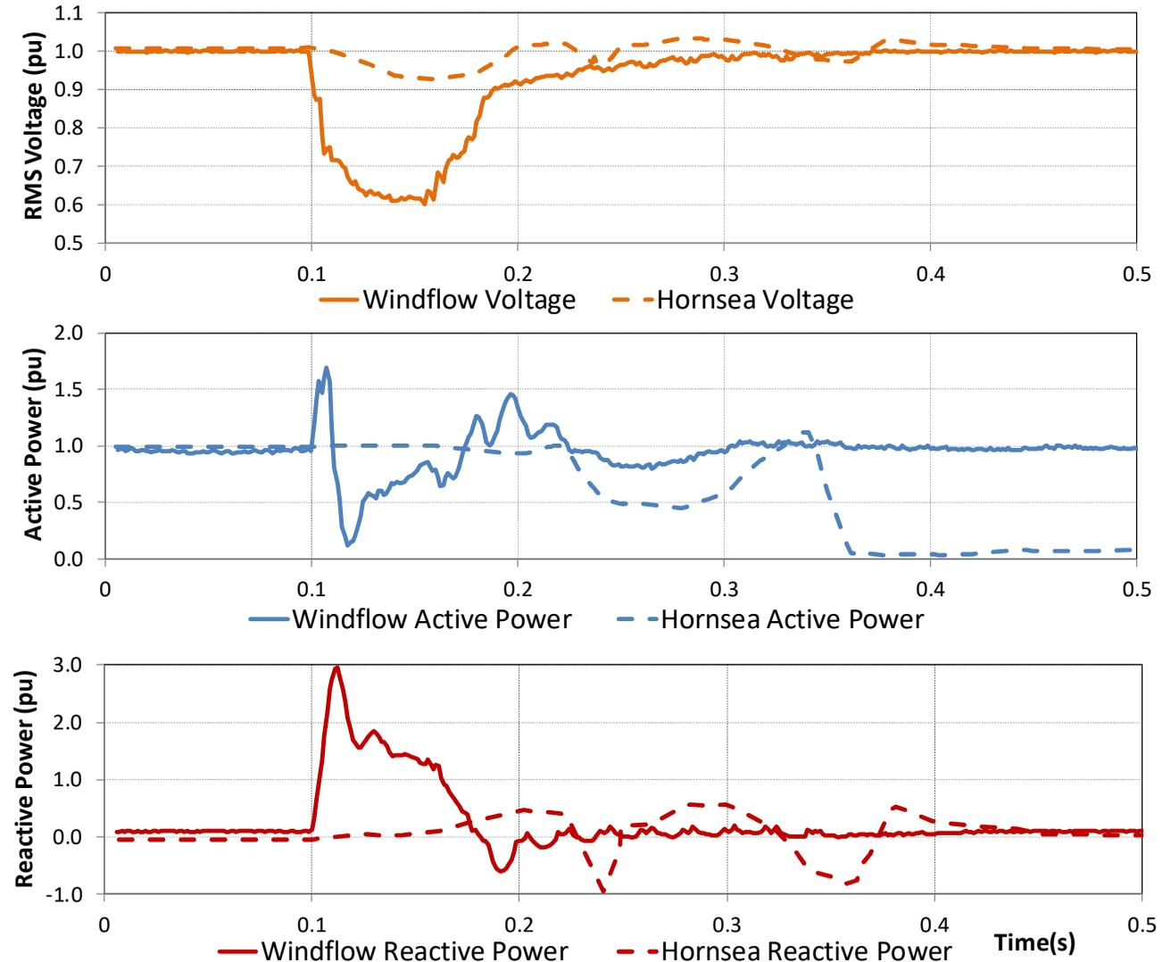
Comparison of fault response of Windflow 500 synchronous turbine at 48 MW wind farm (8/9/2012), and Hornsea 737 MW wind farm (9/8/2019)
