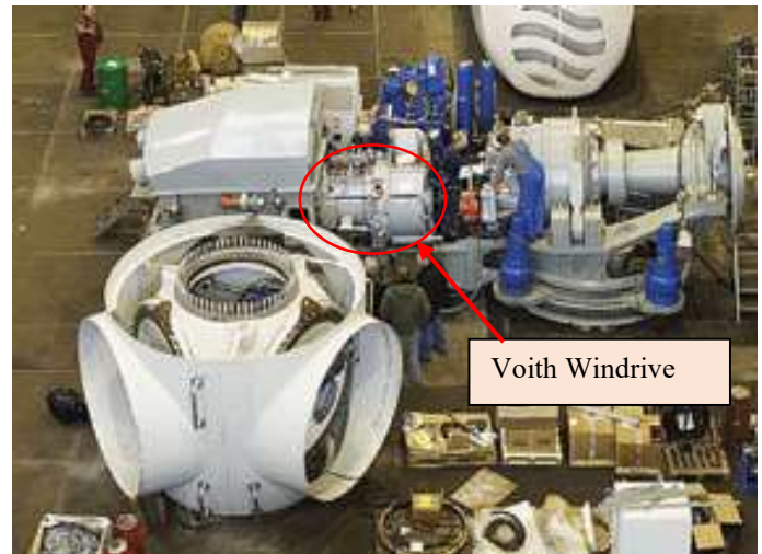
Figure 6 - WinDrive mounted at front of 2 MW generator (Credit: Renewable Energy World [5])
